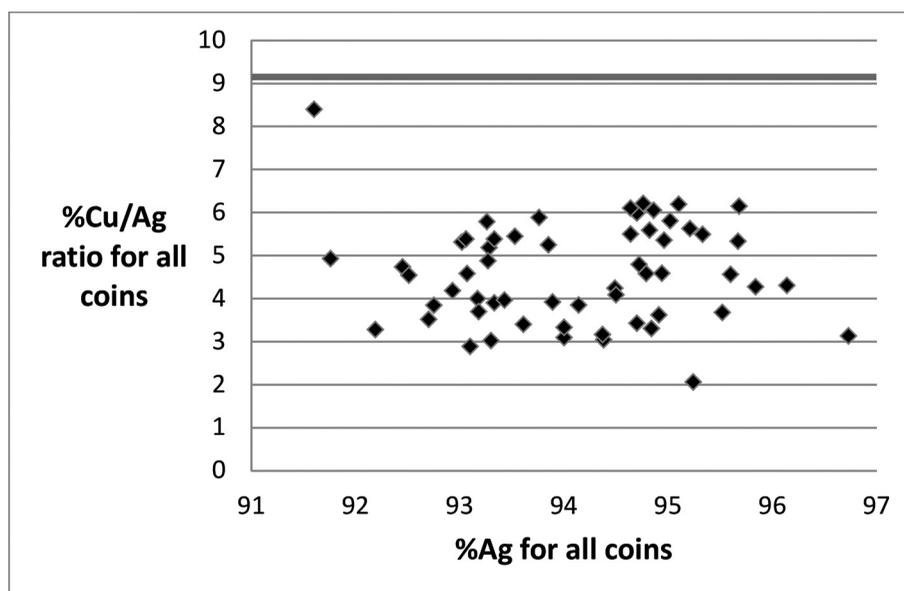
Fig. 2c. Plot of Cu/Ag ratio (in %) vs Ag content (in %)
