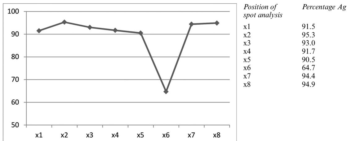
Fig. 1a. Variation of percentage silver content across the section of a 1669 merk on a spot by spot basis from one external surface (position 1) through the core (positions 2–7) to the other external surface (position 8). Composition table (right).
