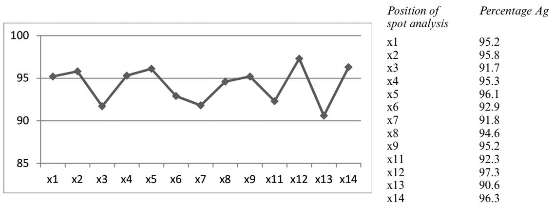
Fig. 1b Variation of percentage silver content across the section of a 1675 eighth dollar on a spot by spot basis from one external surface (positions 1, 2, 12–14) through the core (positions 3–7) to the other external surface (positions 8–11). Composition table (right).
